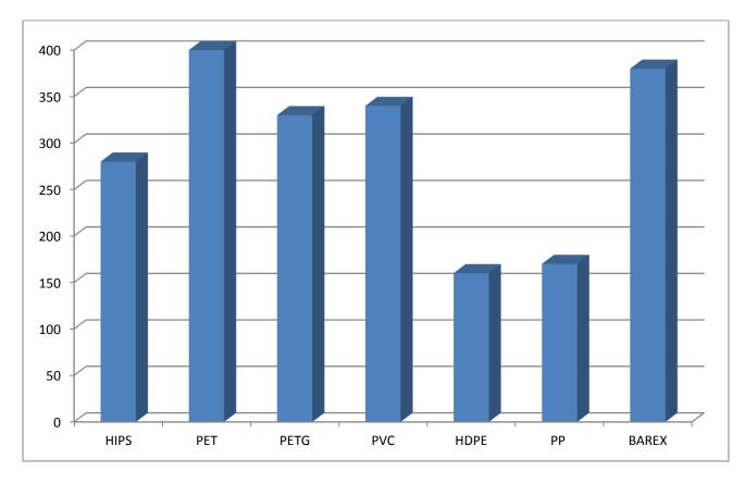
Tensile yield is a measurement of the amount of tension stress a material will withstand before it starts to stretch.
