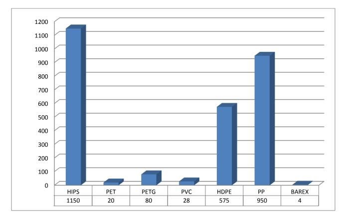
This chart shows the resistance of the material to carbon dioxide  $(CO_2)$  trying to move through it. A low value indicates the material provide a barrier against carbon dioxide migration.
