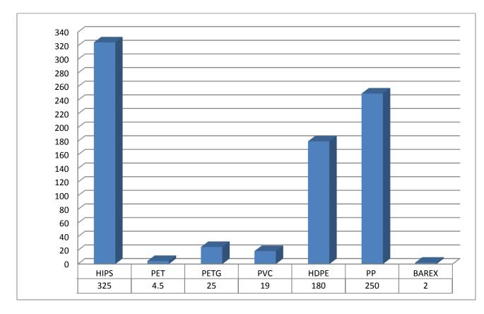
This chart shows the resistance of the material to oxygen  $(O_2)$  trying to move through it. A low value indicates the material provide a barrier against oxygen migration.
