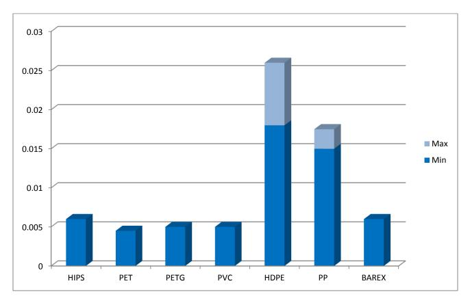
The designer uses mold shrinkage factor to predict how much the plastic will shrink after being formed into the desired geometry.
