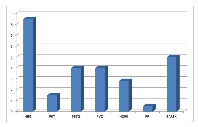
MVTR is a measurement of the resistance of the material to moisture trying to move through it. A low value indicates the material provides a barrier against moisture migration.
