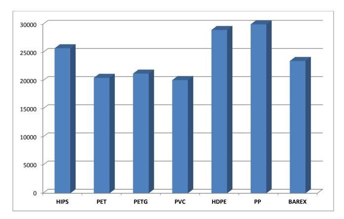
Material yield expresses the amount of surface area one pound of material will cover at a specific thickness, usually one thousandths of an inch. This value is directly proportional to the materials density, but makes it easier to calculate the economy of any given material.
